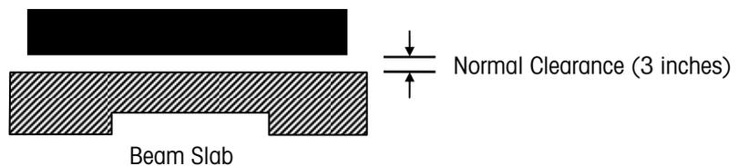
A beam slab is designed to "float" and does not require a deep footer.
