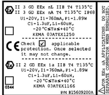
If you install a load cell in a hazardous area, use a permanent marker to place a mark in the check box on the label that indicates the applicable protection (KEMA 03ATEX1250 or KEMA 03ATEX1166). Once the label has been marked, it may not be changed.
