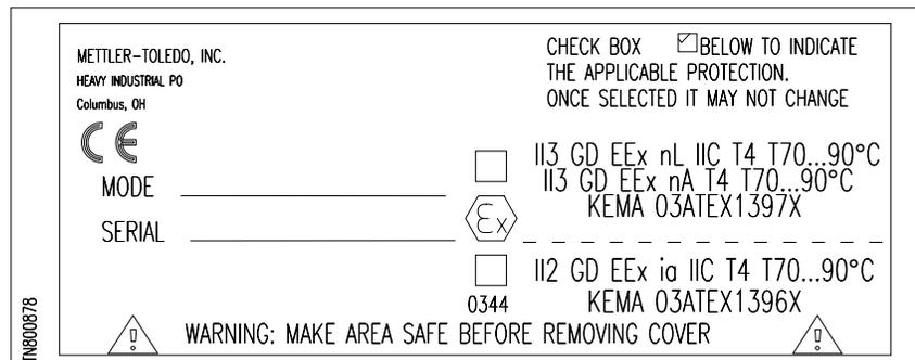
If you install a junction box in a hazardous area, use a permanent marker to place a mark in the check box on the label that indicates the applicable protection (KEMA 03ATEX1396 X or KEMA 03ATEX1397 X). Once the label has been marked, it may not be changed.
