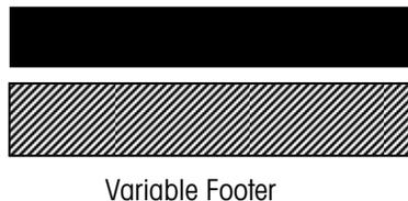
A variable footer design uses separate footers with depths of 2 feet to 6 feet. Connecting "washout" slab is mandatory in some areas.
