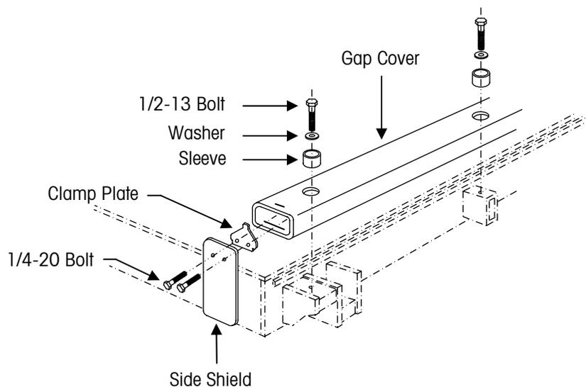
**Figure 5-6: Gap Cover and Side Shield Installation**
