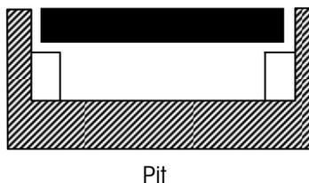
A pit design provides 2 feet or 4 feet of clearance under the scale. It generally requires manholes for access. A deep pit is mandatory in some states.
