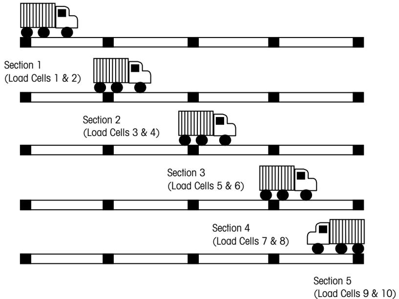
**Figure 7-2: Test Truck Positions for Shift Compensation**
