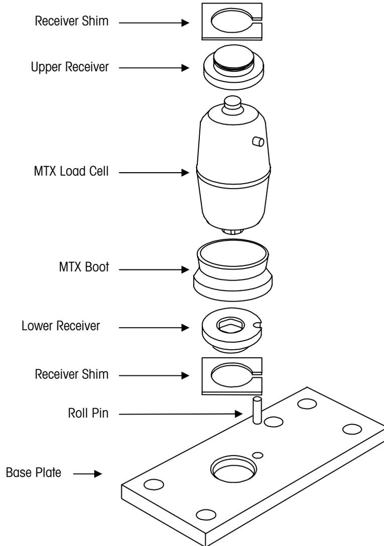
**Figure 5-4: Load Cell Installation**
